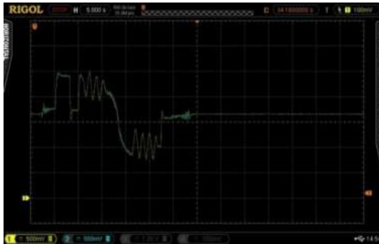
Figure 12 Oscilloscope images of I_{q\_ref} and I_q currents at the system's load changes.
